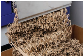
High bulk void fill from waste cartons
